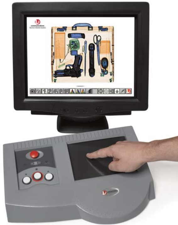
L-3's patented operator interface combines 3-button conveyor control with a touch-sensitive pad that allows continuous heads-up operation using icons displayed on the viewing screen
